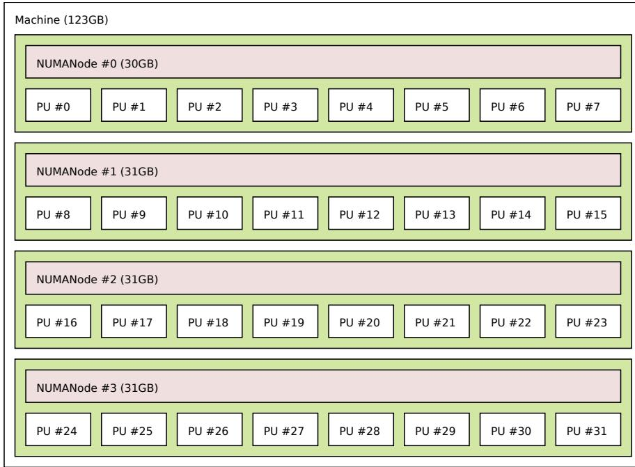
Notice that hwloc only sees half the PUs when SMT is disabled. PU #15, for example, seems to change location from NUMA node #0 to #1. In reality, no PUs "moved" -- they were simply re-numbered when hwloc only saw half as many. Hence, PU #15 in the SMT-disabled picture probably corresponds to PU #30 in the SMT-enabled picture.
