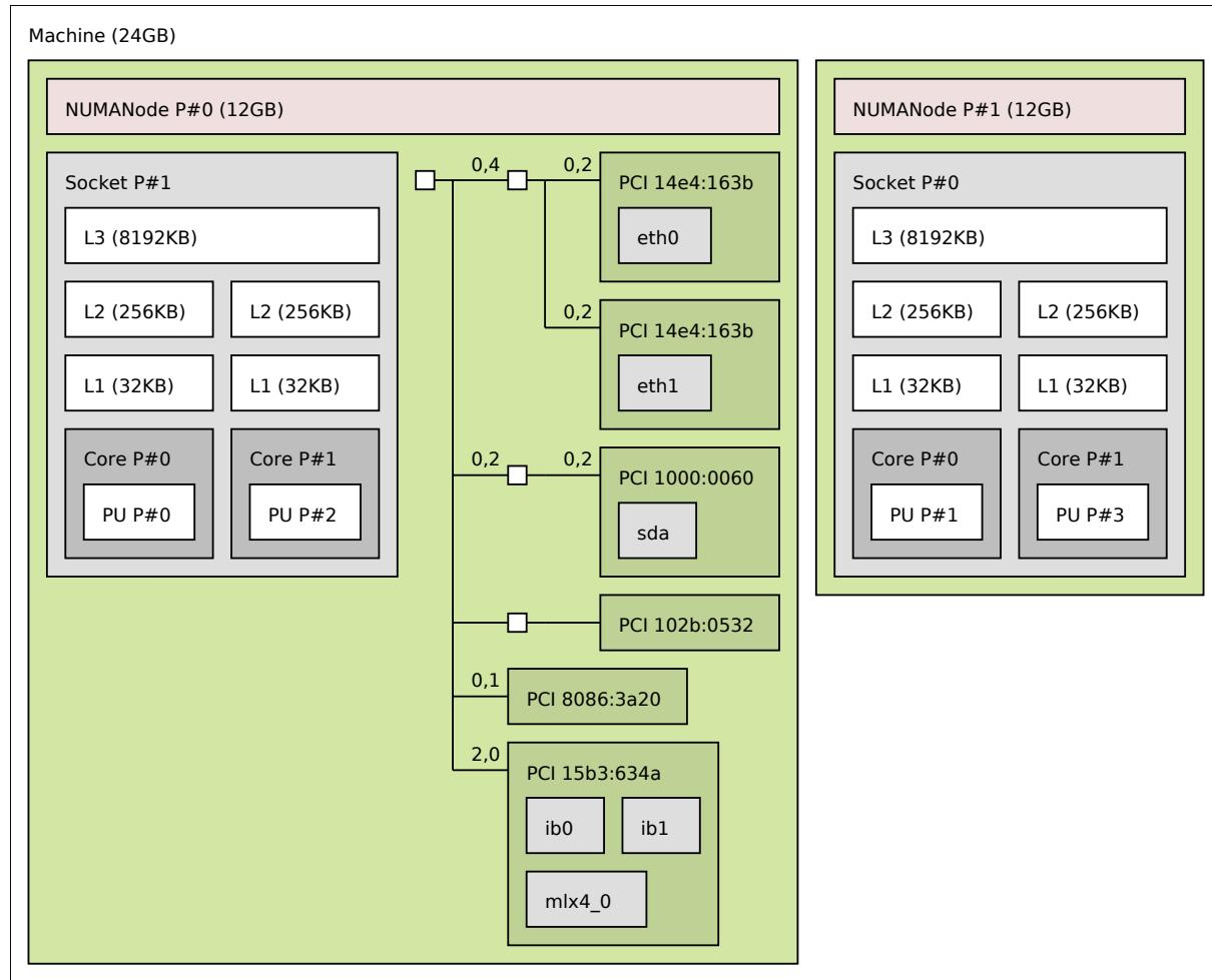
Six interesting PCI devices were discovered. However hwloc found some corresponding software devices (*eth0*, *eth1*, *sda*, *mlx4\_0*, *ib0*, and *ib1*) for only four of these physical devices. The other ones (*PCI 102b:0532* and *PCI 8086:3a20*) are an unused IDE controller (no disk attached) and a graphic card (no corresponding software device reported to the user by the operating system).
