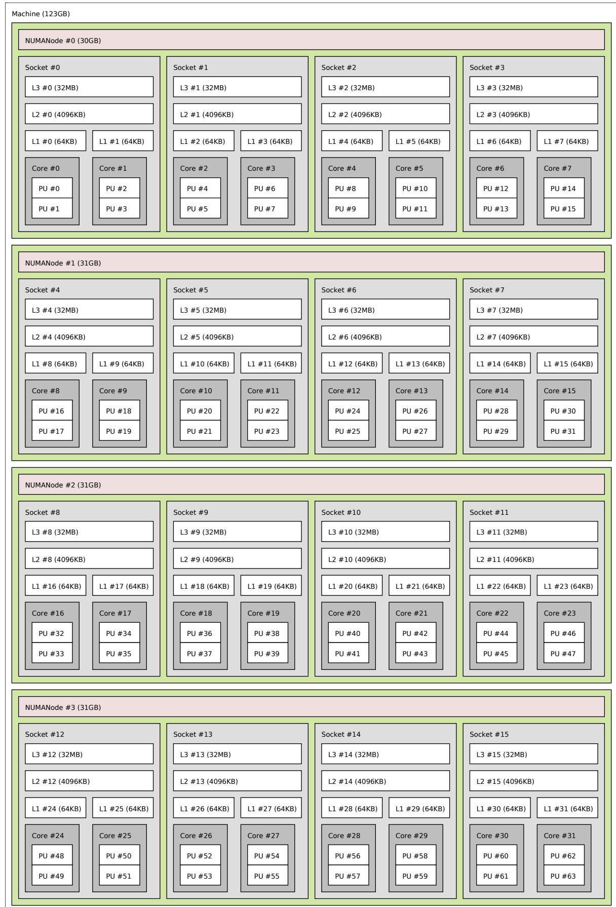
Developers using the hwloc API or XML output for portable applications should therefore be extremely careful to not make any assumptions about the structure of data that is returned. For example, per the above reported PPC topology, it is not safe to assume that PUs will always be descendants of cores.
